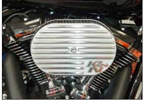
12. Attach cover plate with provided socket head Allen screw.
