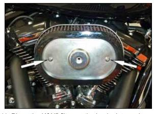
11. Place the K&N® filter on the back plate and attach with the remaining button head screws. NOTE: Apply one drop of provided thread locker to each screw.
