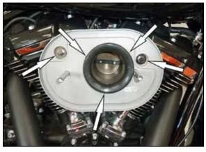
10. Install the filter back plate onto the throttle body and secure first with the throttle body bolts and then with the breather bolts.
