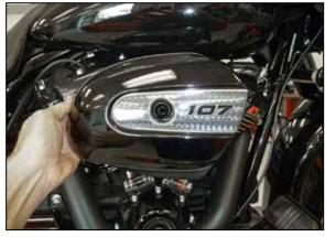
2. Remove air filter cover bolt and air filter cover as shown.
